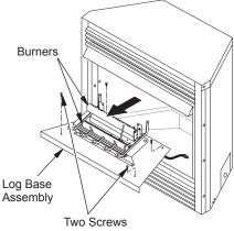
Figure 2 - Removing Log Base Assembly from Fireplace
